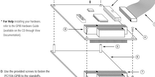
**E**. Plug in the GPIB ribbon cable.
